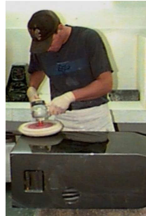
Kevin Crow is polishing and wet sanding, the last of seven steps in the finishing process. Before the seven step process, this Sophia’s surface was similar to the texture of an orange peel. Not only does this process create a glass-like smoothness, it also brings out the speaker’s premium luster.
