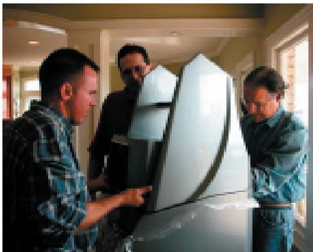
Peter McGrath (right) assists Jeff Fritz in positioning the lower midrange module (LMRM) within Alexandria's wing assembly. The LMRM rests upon the Adjustable Group Delay™ alignment plate.
